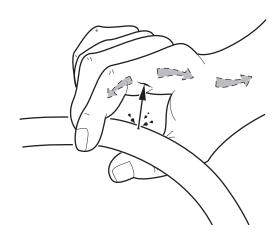
Fluid leaks may not be visible to the naked eye. Use a piece of cardboard to check for leaks, **not** your hand.
