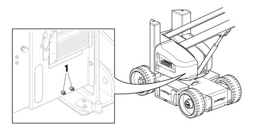
3) Pump the grease gun two to three times as required. Use lithium based (Ep) grease corresponding to DIN 51825 K2K - 20 and ISO L-X-BCHA2. It is also permissible to use equivalent grease with a working temperature between -20°C (68°F) and +120°C (248°F).
