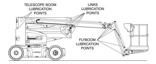
Use a dry PTFE aerosol lubricant spray such as WD40 W/D44394 or equivalent. Apply lubricant spray and allow to penetrate at each of the pivot bush joints identified in the diagram above. Note; there are no grease or lubrication nipples on the pivot bushes.
